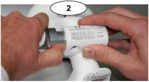
Push in the snap-lock pin of the telescopic handle and insert it into the diagonal joint adapter.
