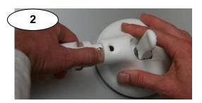
Then push in the snap-lock pin of the angle joint adapter and slide it into the suction head.
