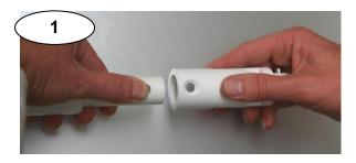
Push in the snap-lock pin of the telescopic handle and insert it into the angle joint adapter.
