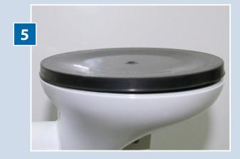
If a handle is attached to a non-porous dense surface for a long period, the rubber gets stretched and slightly curved (Fig. 5).
