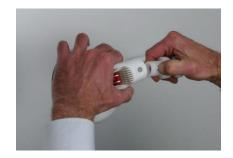
Then press in the quick lock of the cardan joint adapter and push it into the suction head.
