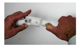
Push the snap pins in (on both sides) of the telescopic bar (fig. 11) and insert the bar into the suction pad housing
